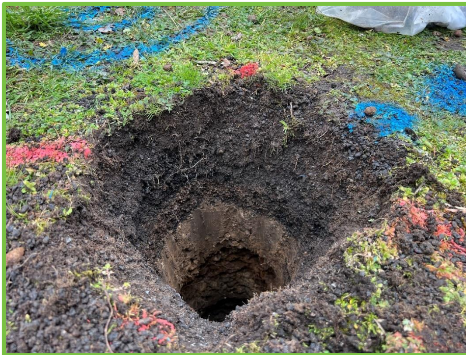
Figure A2. Trial pit investigations (trial pit HP-OB01)
